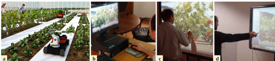
Fig. 8: Human-robot collaboration for increasing the efficiency of robot control in agriculture, (a) teleoperation via simulation environment (Image: Adaptive AgroTech),
