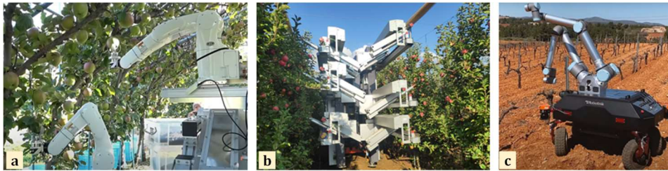
Fig. 1: Multi-robot arms used for increasing efficiency, (a) dual-robot arm for pears and apples harvesting (Image: NARO), (b) apple harvesting machine with multi-robotic arms, (Image: FFRobotics), and (c) integration of a mobile robot with dual-robot arms for grapes harvesting (Image: Robotnik)
