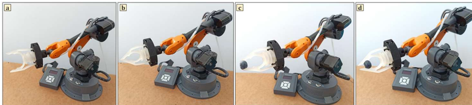
Fig. 4: WLkata Mirobot robotic arm with the custom-designed soft gripper showing (a) extended position, (b) closed position, (c) blueberry grip with the tip, and (d) blueberry grip in locked position for harvesting
