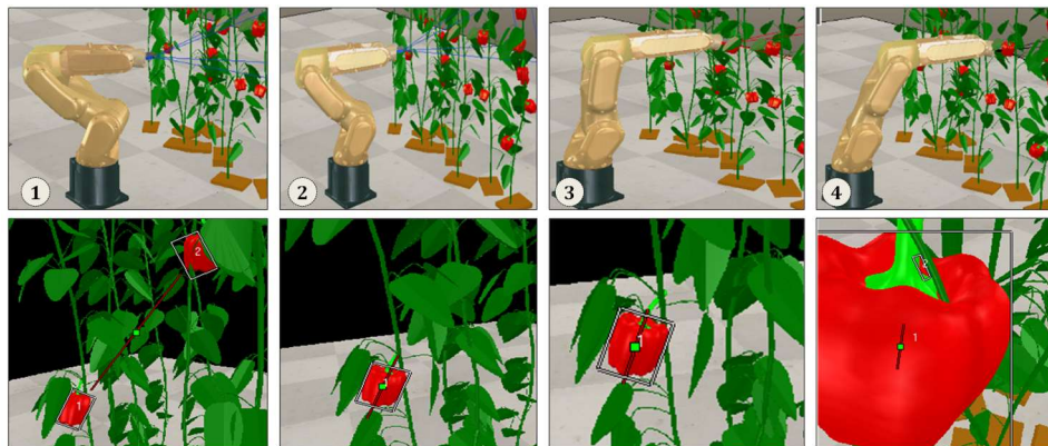
Fig. 4: Simulation of visual servo control experiment with the eye-in-hand configuration and PID Control law on joint angles with feedbacks from image moments. Stability was achieved in 2.5 seconds [Sh18b]
