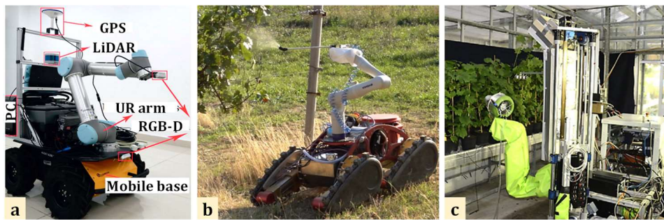
Fig. 7: Examples of robot manipulators with different sensing systems used in weeding, target spraying, and phenotyping, (a) a 6 DoF UR5 robot arm mounted on Husky A200 mobile robot for automated weeding in cornfields [Zh21b], (b) 7-DoF Kinova Gen3 robot arm for target spraying of vineyard [VVK22], and (c) CROPS manipulator for target spraying of grapevines [Ob16]
