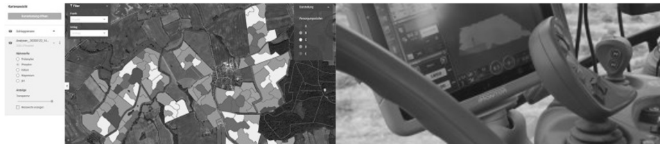
Fig. 1: Left: Predict vegetation levels from satellite images and optimize fertilizer using machine learning. Right: Transfer fertilizer estimations to tractor for precise distribution
