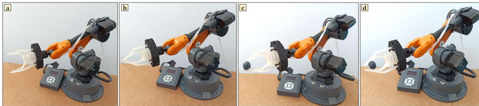
Fig. 4: WLkata Mirrobot robotic arm with the custom-designed soft gripper showing (a) extended position, (b) closed position, (c) blueberry grip with the tip, and (d) blueberry grip in locked position for harvesting
